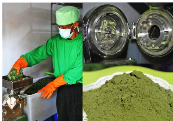
Flouring using stainless steel machine, and packaging with aluminum foil. Level of refinement reached to 200 mesh. Our packaging size of 250 g, 500 g, 1 kg, 5 kg, 10 kg, 20 kg.
