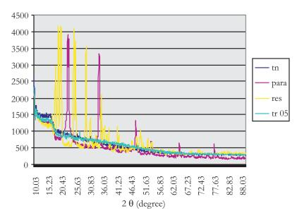
Figure 1 Diffractogram of TRF adhesive and each individual component (T, R, and F)
