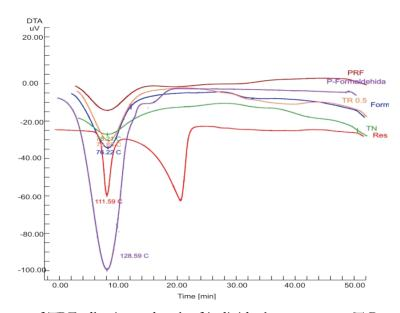
Figure 2. Thermogram of TRF adhesive and each of individual components (T, R, and F) Remarks: tr05= tannin-resorcinol-formaldehyde (TRF) adhesive at mole ratio of T : R : F = 1 :0.5:1; tn = tannin; para/p-Formaldehyde = paraformaldehyde form= formaldehyde; res = resorcinol; PRF = phenol-resorcinol-
