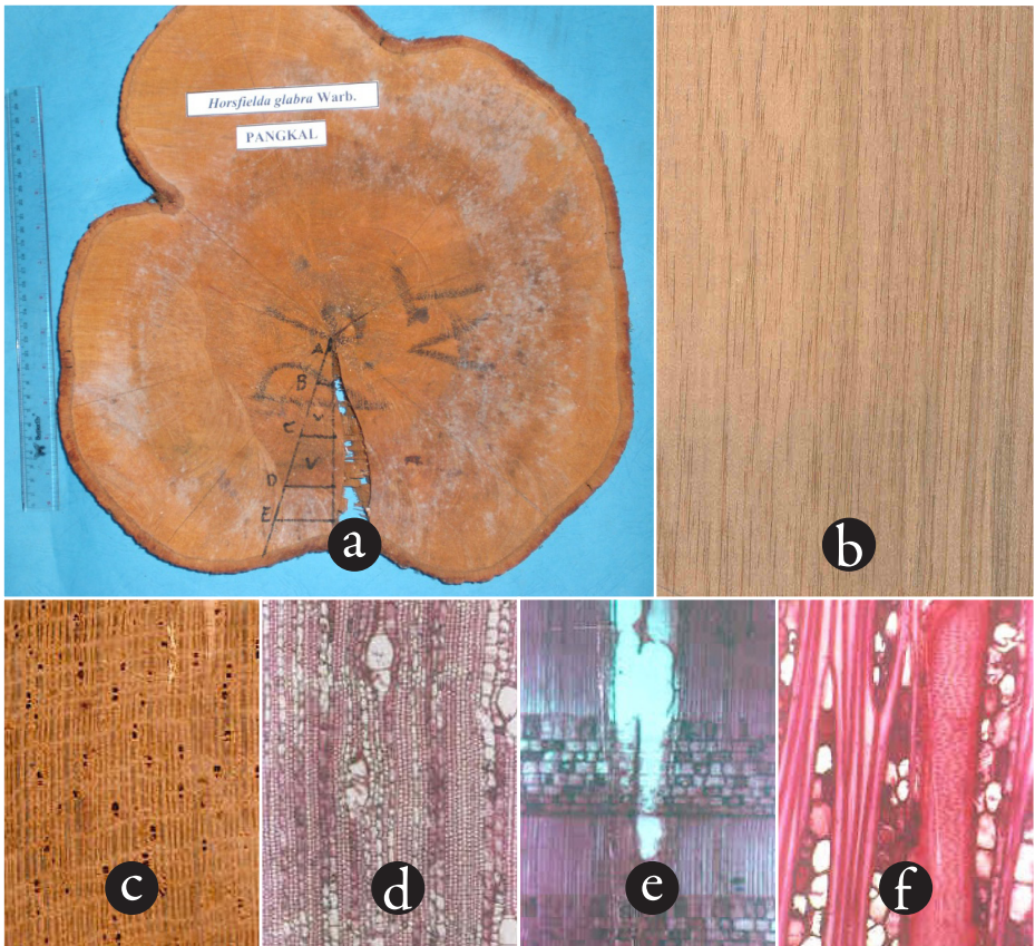
Figure 6. Horsfieldia glabra - Myristicaceae. (a) cross sectional surface of the stem (b) longitudinal surface, x 1 (c) transverse surface (macroscopic), x 10 (d) transverse surface (microscopic), x 40 (e) radial surface, x 100 (f) the alternate and opposite intervessel pits, x 100.
