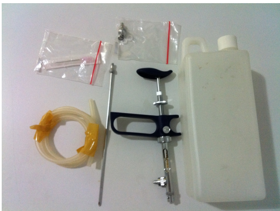
Figure 2. Injection equipment for gaharu liquid inoculant with dosage.
